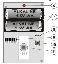
Figure: 6 – red detector activation indicator; 7 – battery; 8 – immunity setting jumper; 9 – production code; 10 – tamper contact; 11 – PIR sensor; <u>Note</u>:
