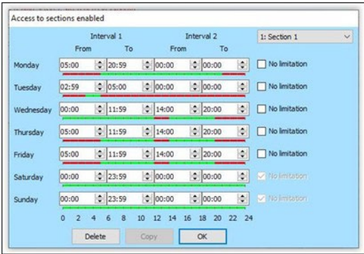
Figure 87 – Access to sections (F-Link)
